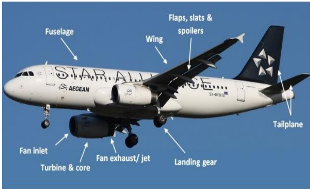
Figure 1.1 Major noise sources of the airframe and engine of a civil aircraft [5]
